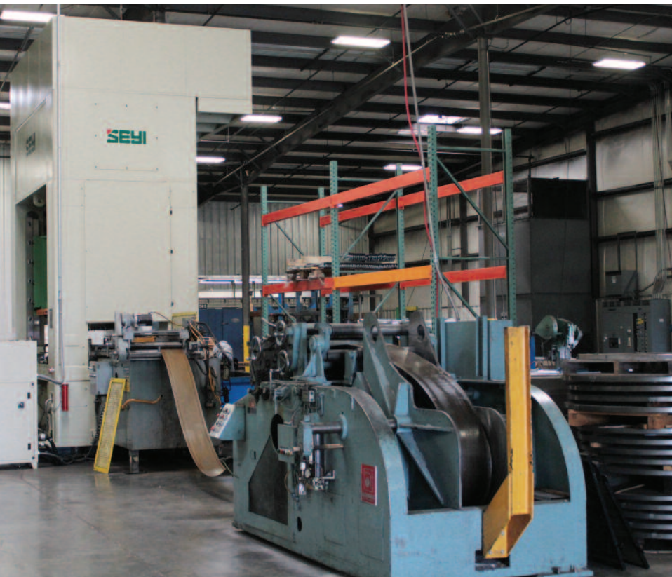
This new Seyi 330-ton press stamps parts for Flexco's line of metal folding steps at 35 to 40 strokes/min., a nice increase compared to the firm's 1950s-vintage press that previously ran at 25 strokes/min.
