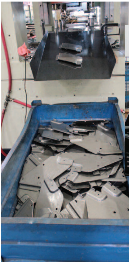
Shown: Stamped folding-step parts exiting Flexco's new press, and assembled steps moving through a production line.
