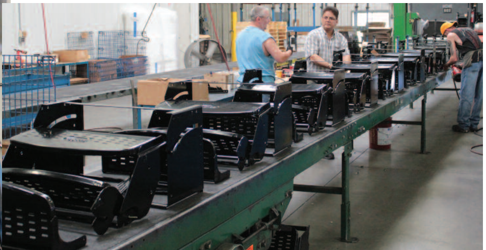
Shown: Stamped folding-step parts exiting Flexco's new press, and assembled steps moving through a production line.
