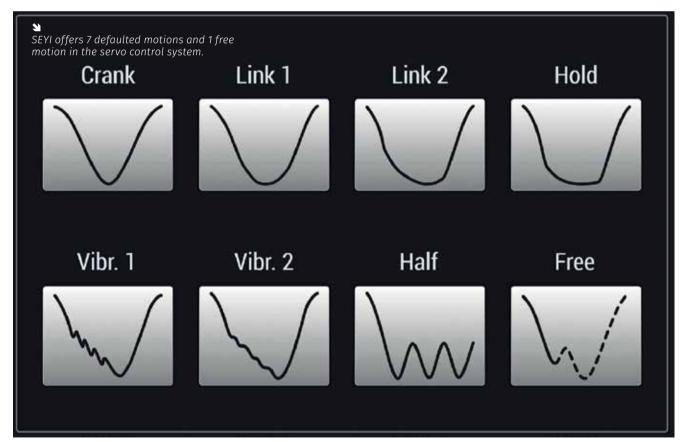
"With an optimised motion control, servo presses can eliminate springbacks or cracks which results in a much lower tool wear rate."
