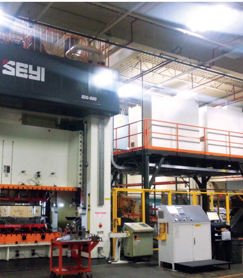
Seyi's servo technology provides low RPMs and high torque, with programmable operation of the slide motion.
